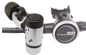
Take the design of our high-performance Dry Air Demand (D.A.D.) first stage. Its unique air-sealed design automatically equalizes pressure without the balancing issues of conventional sealed systems and without letting water inside. No water inside means no silt, sand, or salt inside. No silt, sand, or salt inside means no clogging, abrasion, or corrosion. That means more reliability in more diving conditions. And, less maintenance over the long haul.
